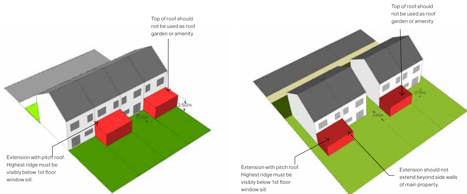
Figure 27: Diagram explaining the basic guidelines for a single rear extension.
