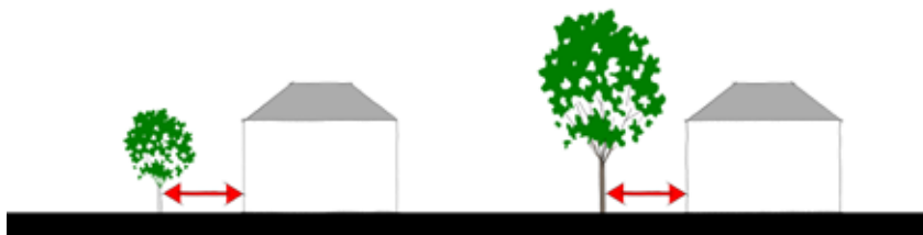
Figure 17: When sitting and planting new trees make sure the future size and canopy of the tree is considered in relation to buildings and adequate distance between them.
